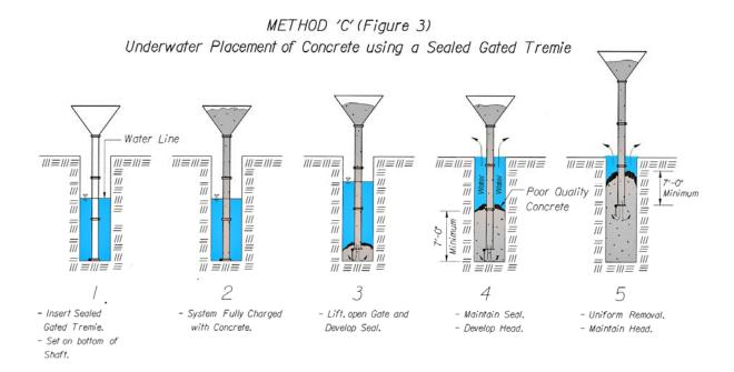
**Method C** (Figure 3): Use a tremie tube, with a sealed gate separating ground water and concrete, to place concrete in the shaft. Fully charge the tremie tube and hopper, then raise the tremie tube by 1 tremie diameter and seal the discharge end of the tremie tube with the fresh concrete.
